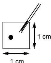
Figure 10-1. Loading a TLC plate.
