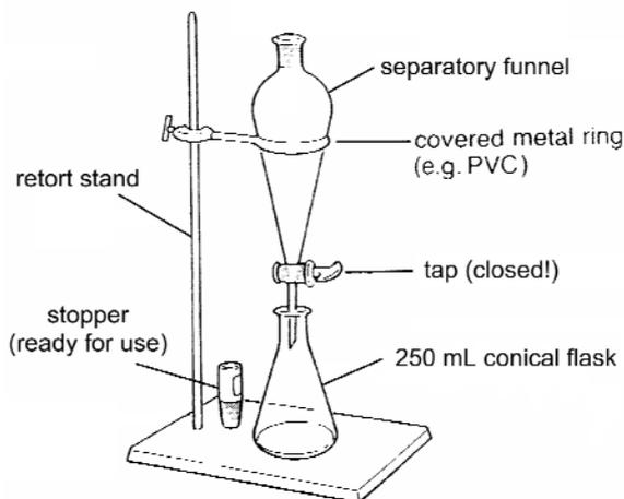
Figure 5-1: Set-up for the separating funnel
