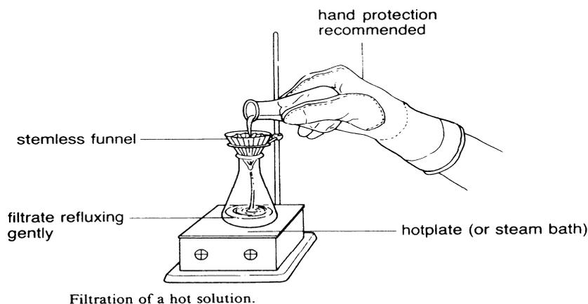
Figure 9-1. Diagram showing the hot filtration of the dissolved compound.
