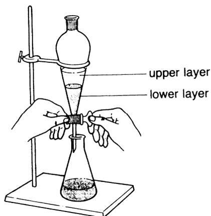
Figure 5-3: The two layers have separated and the lower layer is being removed.
