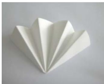
Open it fully, place it in the funnel supported by a retort ring and moisten with a little solvent.
