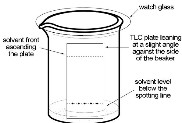
Figure 10-2. Developing a TLC plate.
