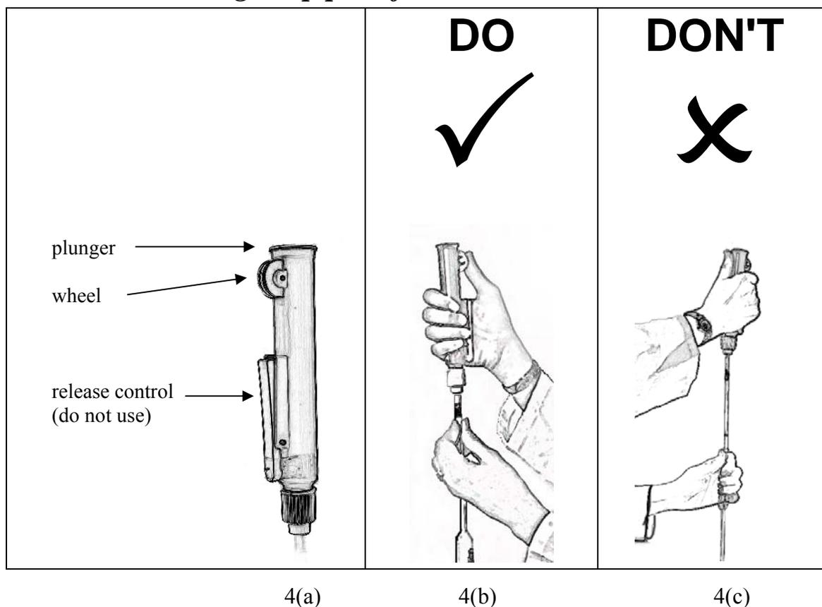
Figure 4-1 Shows a diagram of (a) pipette filler; (b) the correct way to hold and insert a pipette into a pipette filler; (c) an incorrect way to hold and insert a pipette into a pipette filler
