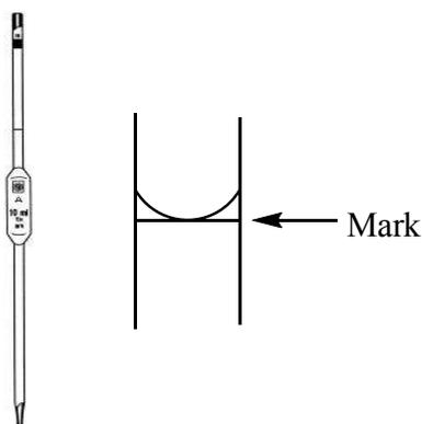
The pipette is a device for delivering a fixed volume of solution. Rinse it with a small amount of water, drain, dry the outside of the tip, and then use the pipette-filler to suck-up a few mL of solution. Use this solution to rinse the entire inside surface of the pipette up to the graduation mark - hold the pipette horizontally and rotate it through at least 360°. Drain. Repeat this rinsing process twice more.
