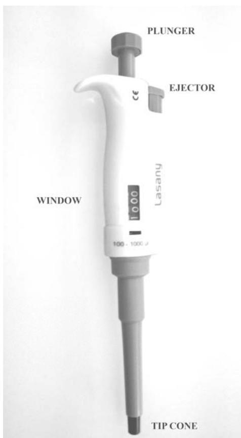
Micropipettes are used for dispensing small quantities of liquids. The Lasany micropipette used in the Boden Laboratories is used to dispense variable volumes of 100  $\mu\text{L}$  - 1000  $\mu\text{L}$ , *i.e.* 0.10 - 1.00 mL.
