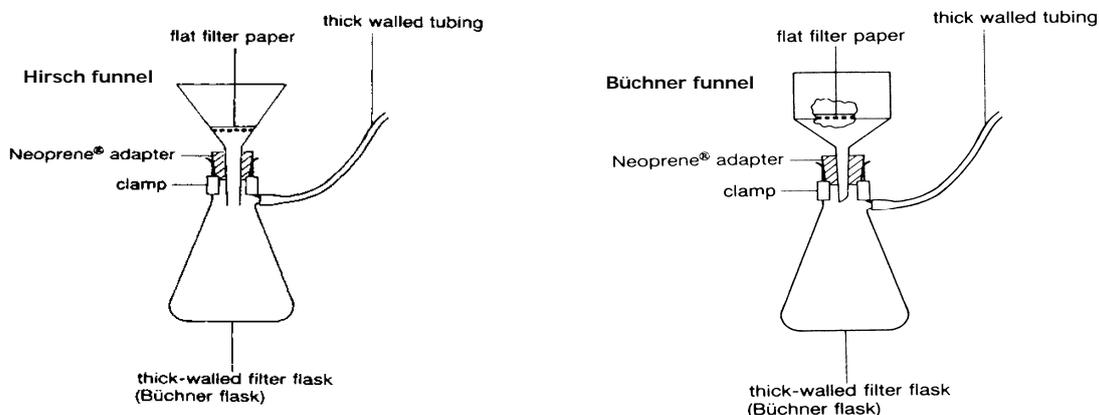
Figure 6-1. Diagram showing how to set up a vacuum filtration.
