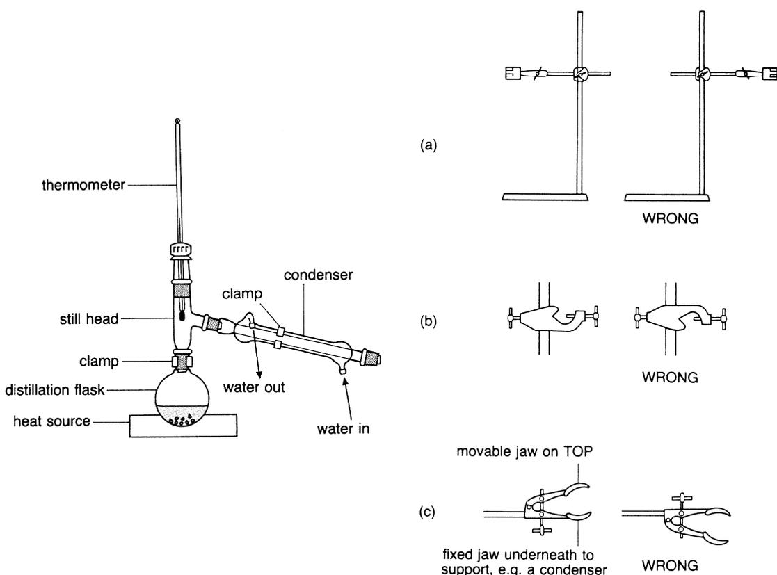
Figure 8-1. Set up of distillation equipment
