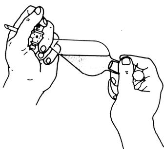
Figure 5-2: How the separating funnel is held.
