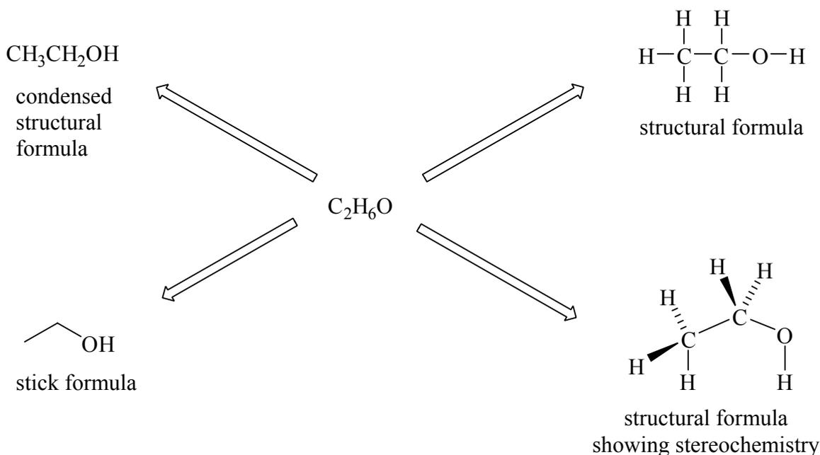
Ethanol is a very simple molecule, but as soon as any complexity is introduced, it is very difficult to comprehend a molecule's structure if all the H atoms are included. So in practice, the stick representation is always used for all but the simplest molecules.
