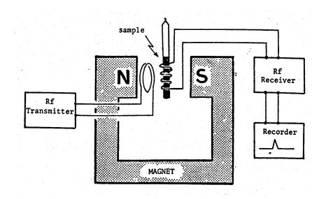
BASIC COMPONENTS OF AN NMR SPECTROMETER
