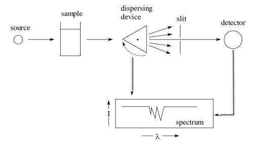
SCHEMATIC DIAGRAM OF A UV OR IR SPECTROMETER
