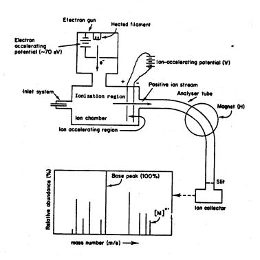
SCHEMATIC DIAGRAM OF AN ELECTRON-IMPACT MASS SPECTROMETER
