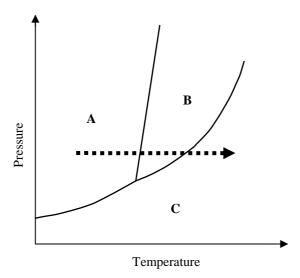
Which phase exists in the fields labelled **A**, **B** and **C**?
