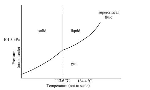
Shown above is the phase diagram for iodine. What are the melting and boiling points of iodine at atmospheric pressure?
