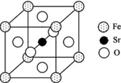
Show the structure is consistent with the formula SrFeO<sub>3</sub> and give the coordination numbers of the Sr, Fe and O atoms.
