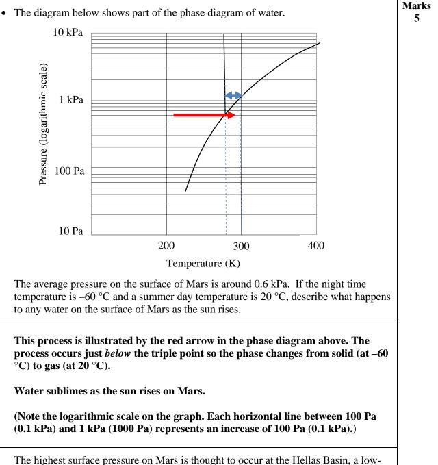
The highest surface pressure on Mars is thought to occur at the Hellas Basin, a lowlying area created by the impact of a large asteroid. If the pressure in this region is 1.2 kPa, use the phase diagram to estimate the temperature range in which liquid water will occur. Show your working on the phase diagram.
