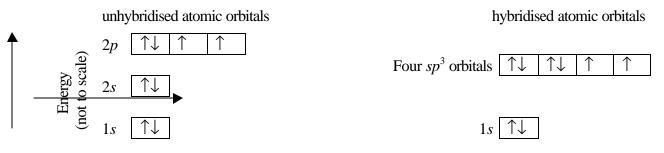
The 2*s*,  $2p_x$ ,  $2p_y$  and  $2p_z$  orbitals of the oxygen atom undergo a mixing process called hybridisation to produce four equivalent  $sp^3$  hybrid orbitals. Two of these orbitals already contain 2 electrons (the non-bonding pairs on the oxygen). Each of the other two  $sp^3$  orbitals that contain 1 electron can overlap with the 1*s* orbital of a H atom to form a  $\sigma$ -bond.
