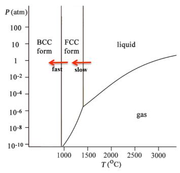
Fast cooling to room temperature does not allow the atoms to re-arrange; they are stuck in the FCC form as considerable re-arrangement is needed to turn this in the BCC form.
