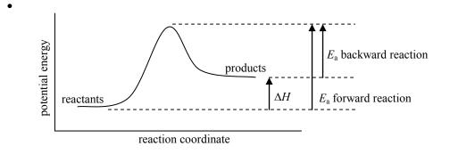
The backward reaction would be faster as it has a lower activation energy.
